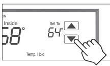
**Press** • or • to adjust the end time of the hold. If end time is not adjusted, the Temporary Hold will end at the start of the next event.
