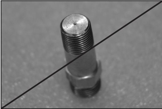
Former stainless steel orifice with 0.020 in. (0.51 ml) hole.
