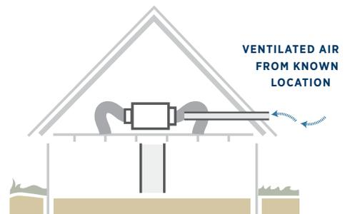
Outdoor air is delivered from a safe location, not passing through the walls.
