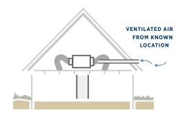
Outdoor air is delivered from a safe location, not passing through the walls.
