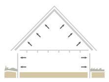
Positive pressure eliminates safety concerns from combustible appliances backdrafting and is easy to measure (CFM).
