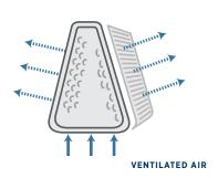
Ventilated air is delivered to the air conditioning evaporator coil to remove moisture.
