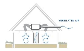
Aprilaire ventilators utilize existing HVAC ducting systems to deliver air throughout the home.
