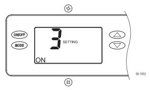
The UP and DOWN arrow buttons allow the dryness setting to be set from 1 to 7. Use the ON/OFF button to turn the dehumidifier ON or OFF.
