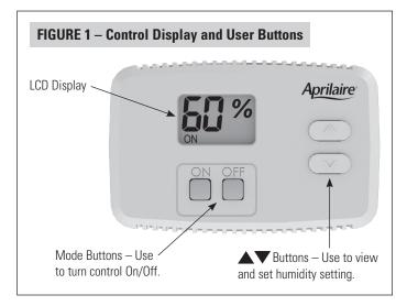
**Energy Savings Tip #1:** Adjust the setting to be as high as is comfortable to reduce dehumidifier run time – if it feels clammy or smells damp or moldy lower the setting. To save energy, turn the dehumidifier control OFF when you open your windows just as you would with air conditioning.
